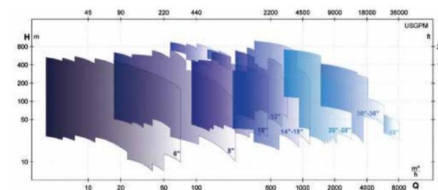
Radial & semi-axial impeller working ranges (50 Hz)
